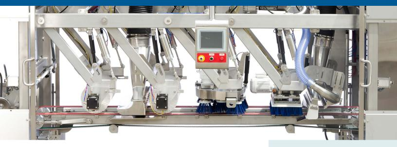
The Bundy/FME Continuous Pan Cleaner continuously moves pans through a multi-stage cleaning process to remove protein washes, seeds, and other loose toppings.\*
