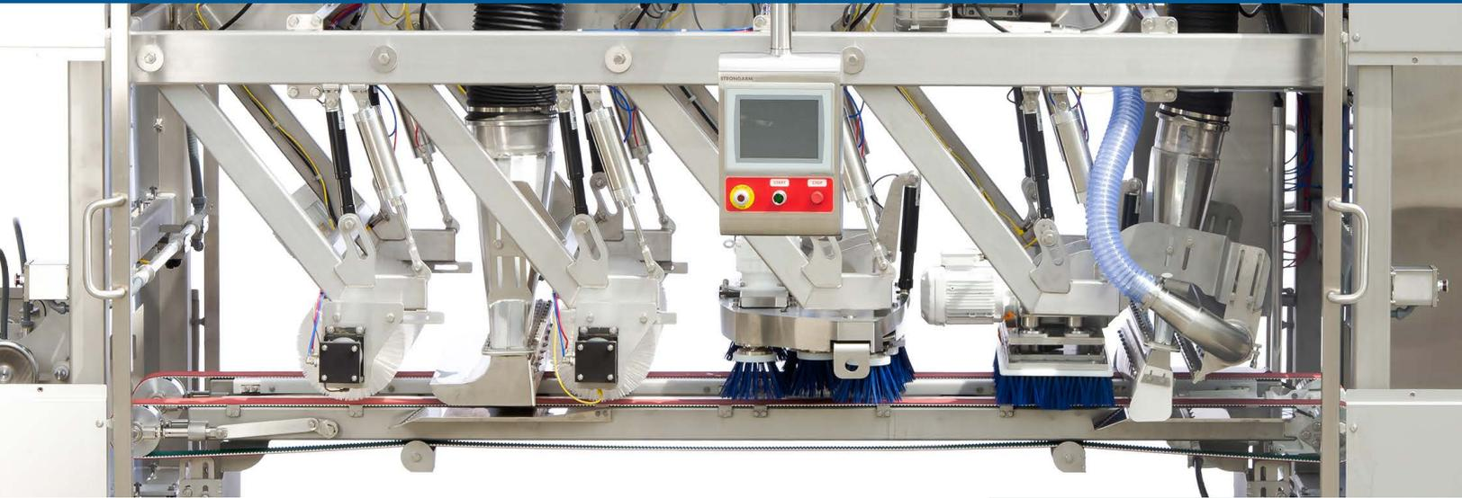
*The Bundy/FME Continuous Pan Cleaner continuously moves pans through a multi-stage cleaning process to remove protein washes, seeds, and other loose toppings.\**
